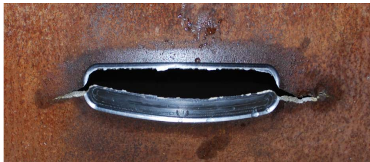
Fig. 4: Corroded pipe after burst test [ 7 ]
