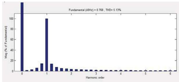
Figure9. FFT Analysis of current ripple
