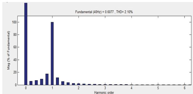
Figure10. FFT Analysis of voltage ripple
