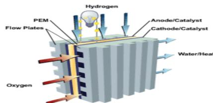
Figure2. Structure of proton exchange membrane
