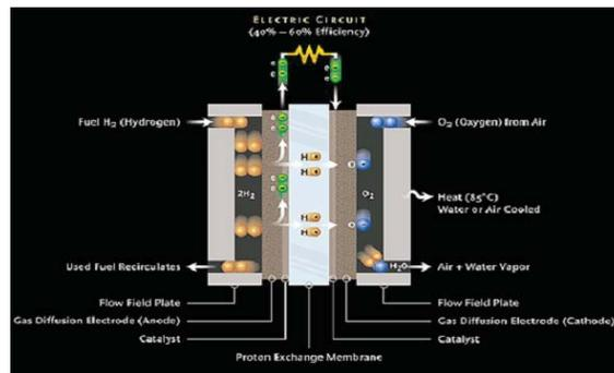
Figure1. Basic operation of PEMFC
