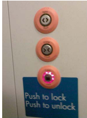
Fig. 2 Automatic door locking system in British trains
