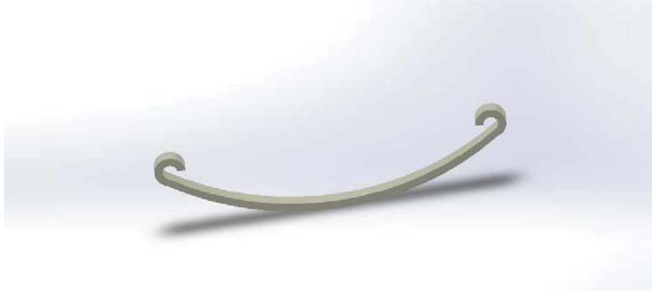
Fig 4. 3D Model of Mono Leaf Spring Using Solidworks
