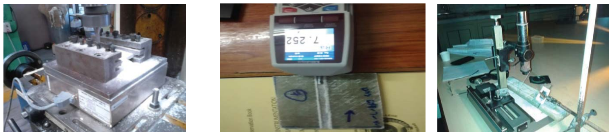
Fig 1. (a) Machining of GFRP laminate plate is properly fixed in machining center by special designed fixture (b). Measurement of surface roughness by Mitutoyo Talysurf (c). Measurement of delamination damage using Travelling Microscope
